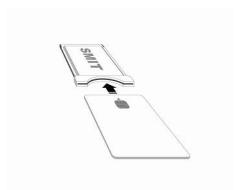
2. Insert the CAM into the IRD or monitoring equipment correctly. Please refer to the following figure. If the CAM is inserted properly, the TV screen will show CICAM initialization information.
